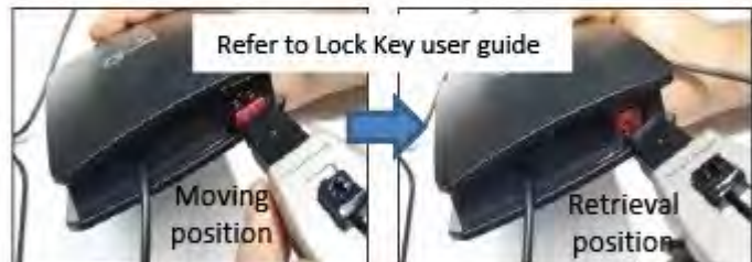
1 Remove USB Port Locks on sides using Lock Key
