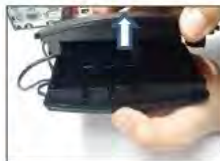
4 Lift Link Lock cover in the direction of arrow
