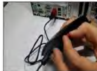
10 Align cover and base to install USB Port Lock
