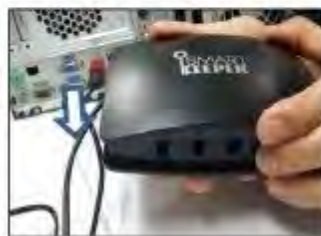
3 Slide Link Lock cover in the direction of arrow
