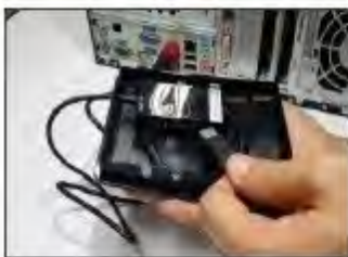
5 Connect desired USB devices to USB hub
