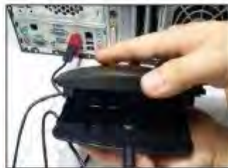
6 Align notch on the cover with notches on base
